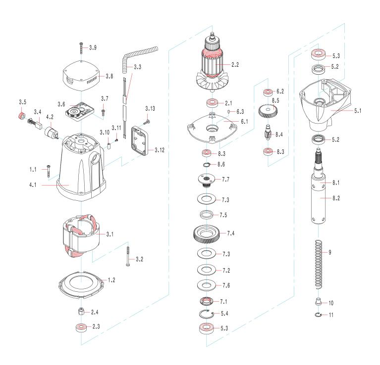
Component parts of motor and gearbox RD23661 (110v) & RD23663 (230v)
