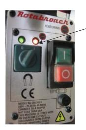
Indicator turns orange when too much pressure is added on the cutter. Will turn Red and cut power to motor if machine is given too much force for the motor to cone with.
