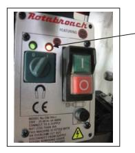
Indicator turns orange when too much pressure is added on the cutter. Will turn Red and cut power to motor if machine is given too much force for the motor to
